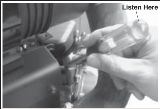
Figure 5B-17. Checking Injectors.
